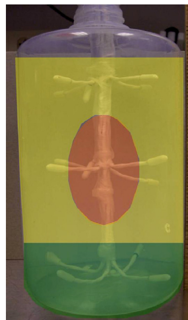
Fig. 1. Temperature sensor array in a 2-L Teflon bottle containing 1.7 L of a buffer composed of 20 mM histidine, 10% sucrose, and 0.02% (w/v) Polysorbate 20 at pH 6.0. Sensors were laid out to measure temperature at the walls on four sides, in the center, at the top, middle, and bottom of the bottle.
